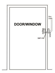
Mount contact on side or top of door or window frame (not on hinge side.)
