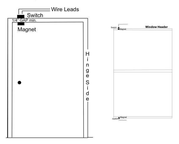
Surface mount switch at top or side (NOT on hinge side) of door or hinged window frame On double hung window, surface mount the switch at top, side or bottom of window frame Surface mount the magnet parallel to the switch
