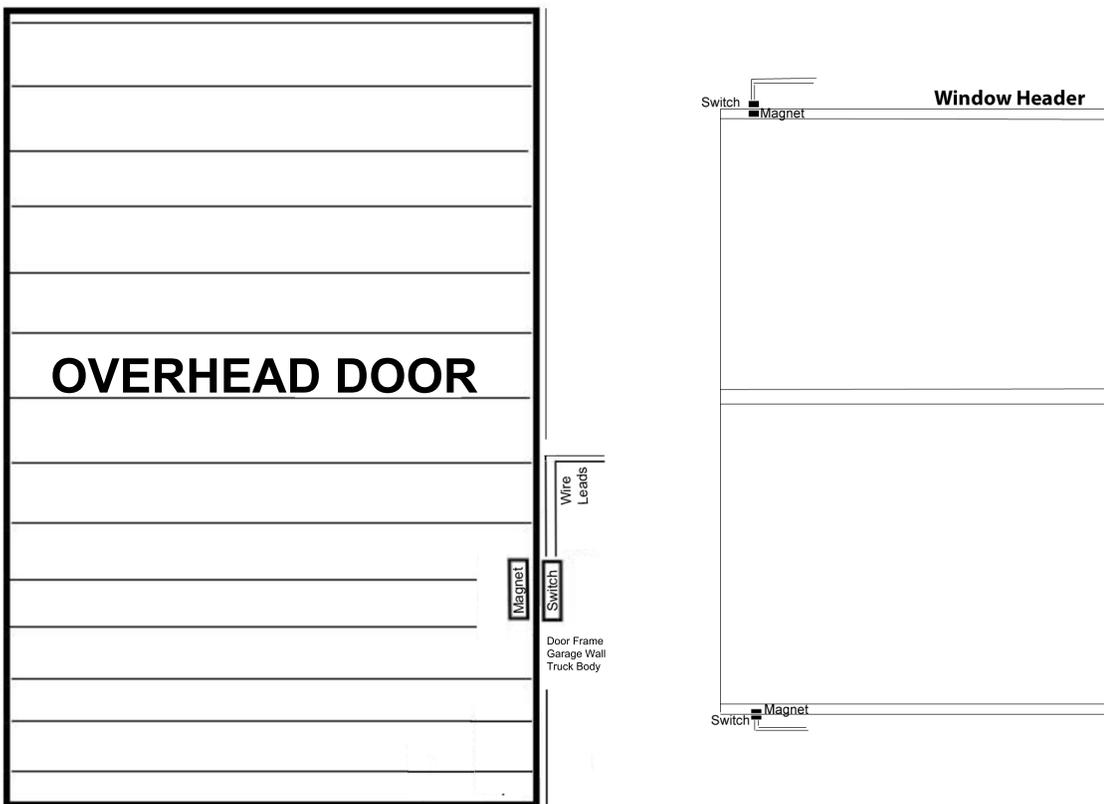
Surface mount switch on top or side of door or window frame, on garage wall or truck body
