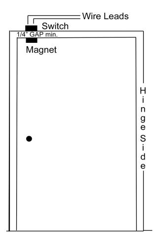
Drill 3/8" hole in window or door frame (NOT on hinge side) to mount the switch Drill 3/8" hole in window or door to mount the magnet Make sure Gap is not less than 1/4" between switch and magnet Insert leads from alarm circuit under terminals NOT for use with Steel doors and windows
