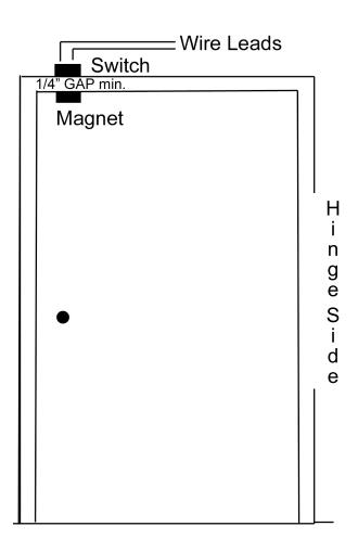
Drill 3/4" hole in window or door frame (NOT on hinge side) to mount the switch Drill 3/4" hole in window or door to mount the magnet Make sure Gap is not less than 1/4" between switch and magnet Insert leads from alarm circuit under the switch terminals Designed for use with Steel, Wood and other door and window materials
