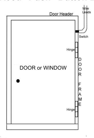
ON HINGE SIDE of door or window frame drill a 3/4" hole for the switch Closing door or window compresses Button Ball into contact shell deactivating alarm \*\* When the door or window opens the button ball extends and the alarm is activated \*\* For TANE-22 splice wire leads into alarm circuit
