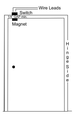
Drill 1/4" hole in window or door frame (NOT on hinge side) to mount the switch Drill 1/4" hole in window or door to mount the magnet Make sure Gap is not less than 1/4" between switch and magnet Splice leads from switch into alarm circuit NOT for use with Steel doors and windows
