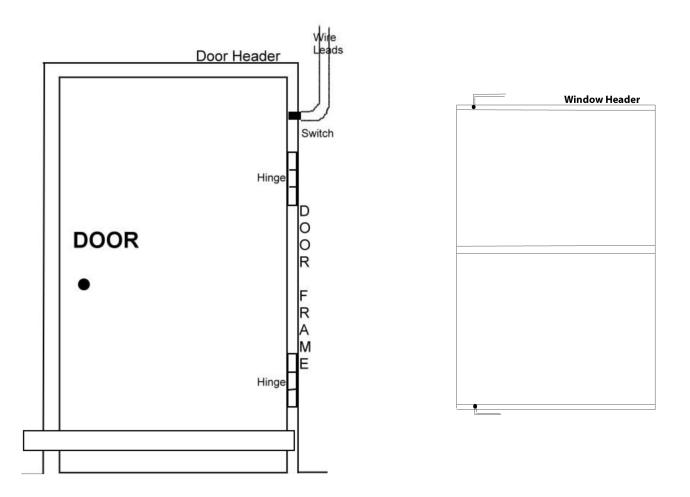
Drill 3/8" hole ON HINGE SIDE of door frame or hinged window to mount switch\* For double hung windows drill 3/8" hole in top or bottom of window channel to mount switch\* Splice wire leads from switch into alarm circuit
