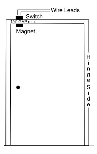
Drill 3/8" hole in window or door frame (NOT on hinge side) to mount the switch Drill 3/8" hole in window or door to mount the magnet Make sure Gap is not less than 1/4" between switch and magnet Splice leads from switch into alarm circuit NOT for use with Steel doors and windows
