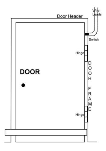
Drill 3/4" hole ON HINGE SIDE of window or door frame to mount switch\* Splice wire leeds from switch into alarm circuit
