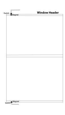
Surface mount switch at top or side (NOT on hinge side) of door or hinged window frame On double hung window, surface mount the switch at top, side or bottom of window frame Surface mount the magnet parallel to the switch
