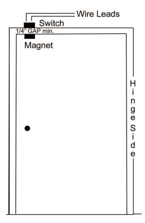
Drill 1" hole in window or door frame (NOT on hinge side) to mount the switch
