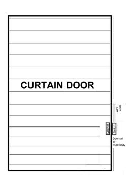
Mount contact on left or right side of curtain door using reversible mounting assembly.
